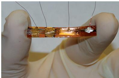
**Electrifying:** A fiber-based hybrid nanogenerator for simultaneous or independent harvesting of mechanical and biochemical energy is presented. The hybrid system consists of a nanogenerator (FNG) and a biofuel cell (FBFC) and provides a peak output of 3.1 V and 200 nA. It also serves as a self-powered sensor for the quantification of pressure variations.
