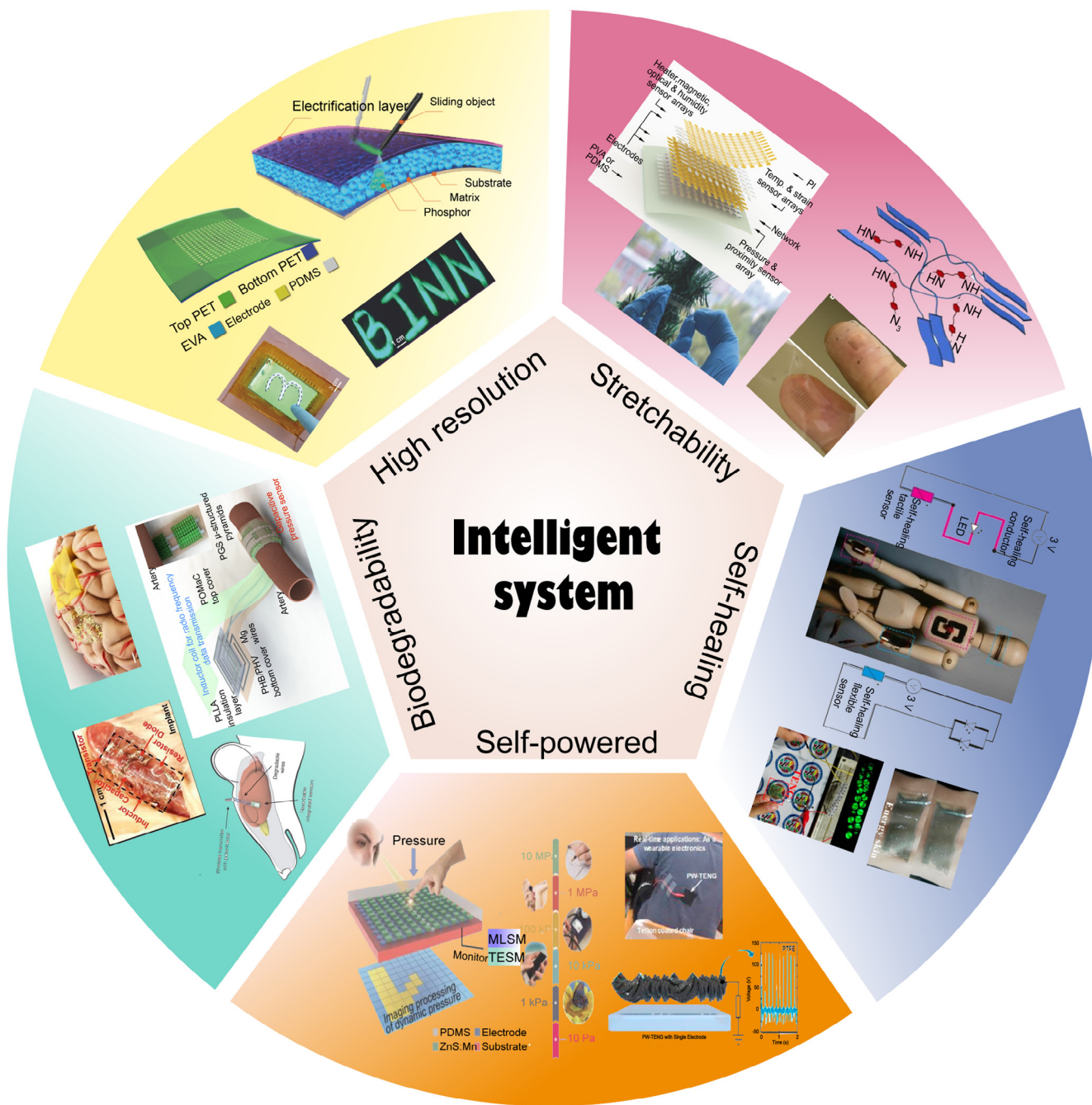
Fig. 1. (Color online) High performance of different tactile sensors applied in intelligent systems. High resolution: a tactile sensor matrix was used for visualized sensing and real-time tactile mapping. Reprinted with permission from Refs. [11,12], Copyright © 2016 Wiley-VCH. Stretchability: tactile sensors based on flexible materials or stretchable structures were used for sensing a variety of stimuli, such as temperature, humidity and stress. Reprinted with permission from Refs. [13–15], Copyright © 2018 Wiley-VCH, © 2018 Springer Nature. Self-healing: tactile sensors can repair themselves because of the interaction between the special covalent bonds or supramolecular bonds, which can extend the service life of tactile sensors. Reprinted with permission from Refs. [16,17], Copyright © 2012, Springer Nature, © 2018 American Chemical Society. Self-powered: nanogenerators, as tactile sensors based on the piezoelectric or triboelectric effect, were used for tactile perception without an external energy source. Reprinted with permission from Refs. [18,19], Copyright © 2017 Wiley-VCH, © 2018 Elsevier. Biodegradability: tactile sensors based on natural or synthetic materials, such as silk protein and PLGA, can be implanted in the body, and they degrade under certain conditions. Reprinted with permission from Refs. [20–23], Copyright © 2012 AAAS, © 2016, 2019 Springer Nature, © 2017 National Academy of Sciences.
